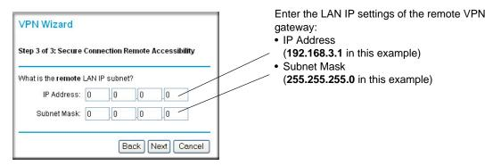
Figure 5-26: Secure Connection Remote Accessibility
